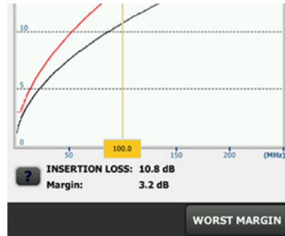
Figure 2. Measured Insertion Loss and limit for 450 foot Type 734 cable.
