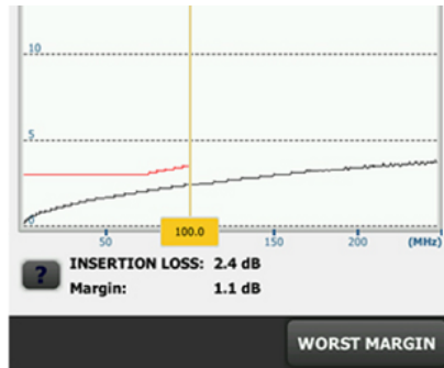
Figure 1. Measured Insertion Loss and limit for 100 foot Type 734 cable.
