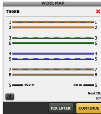
Wiremap – shows distance to fault, break and short
